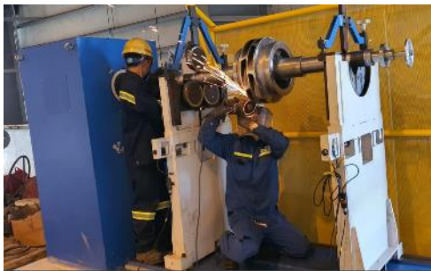
Balancing for pump impeller
