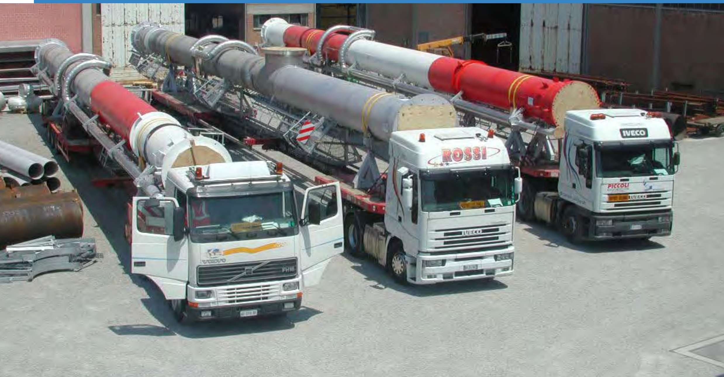
Flare Risers ready for shipping out
