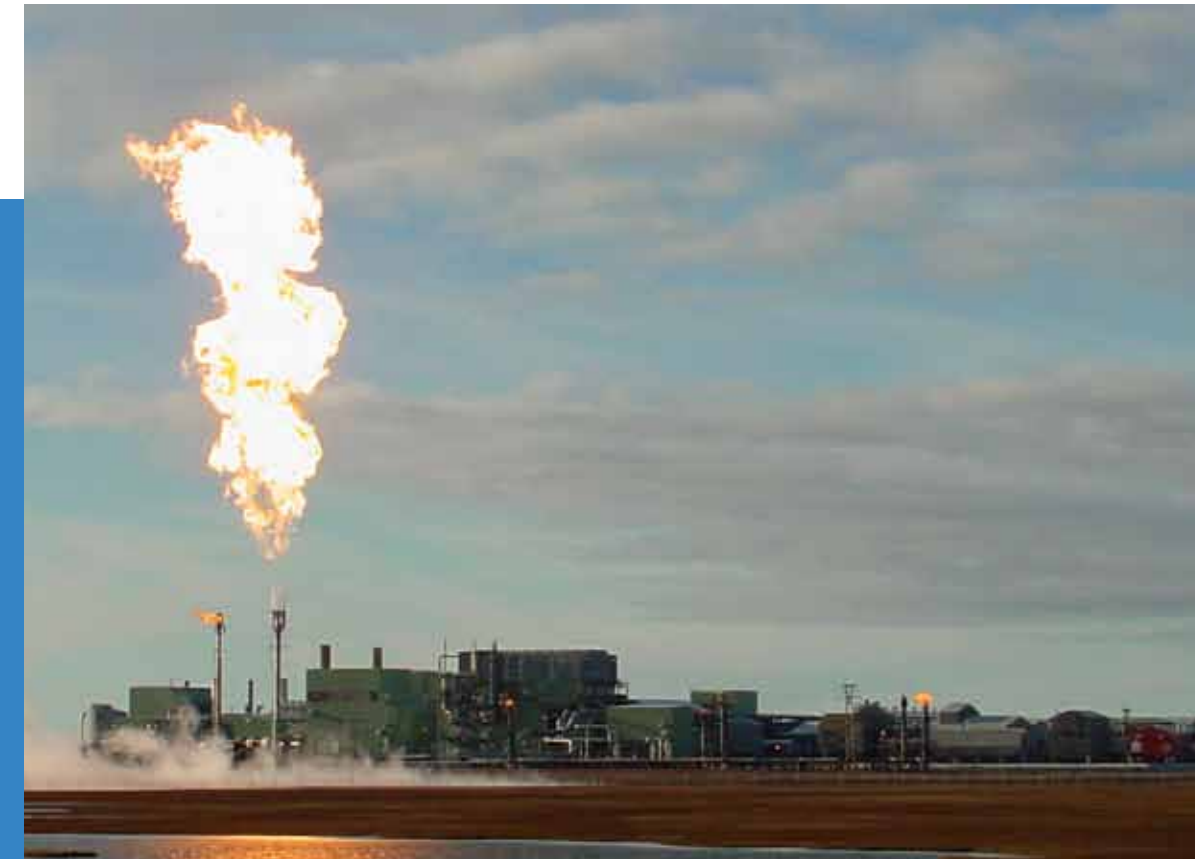
CSF-7-14 Flare Tip Being tested at maximum flow in Alaska
