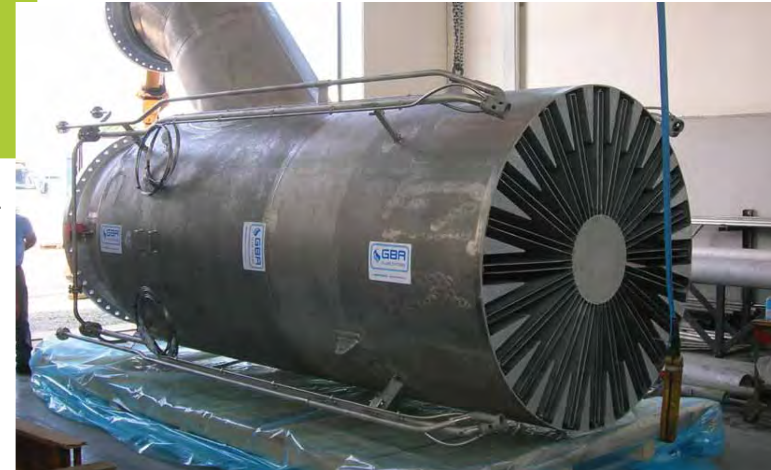
CAF-36-30 Air Assisted Flare Tip Olefins plant
