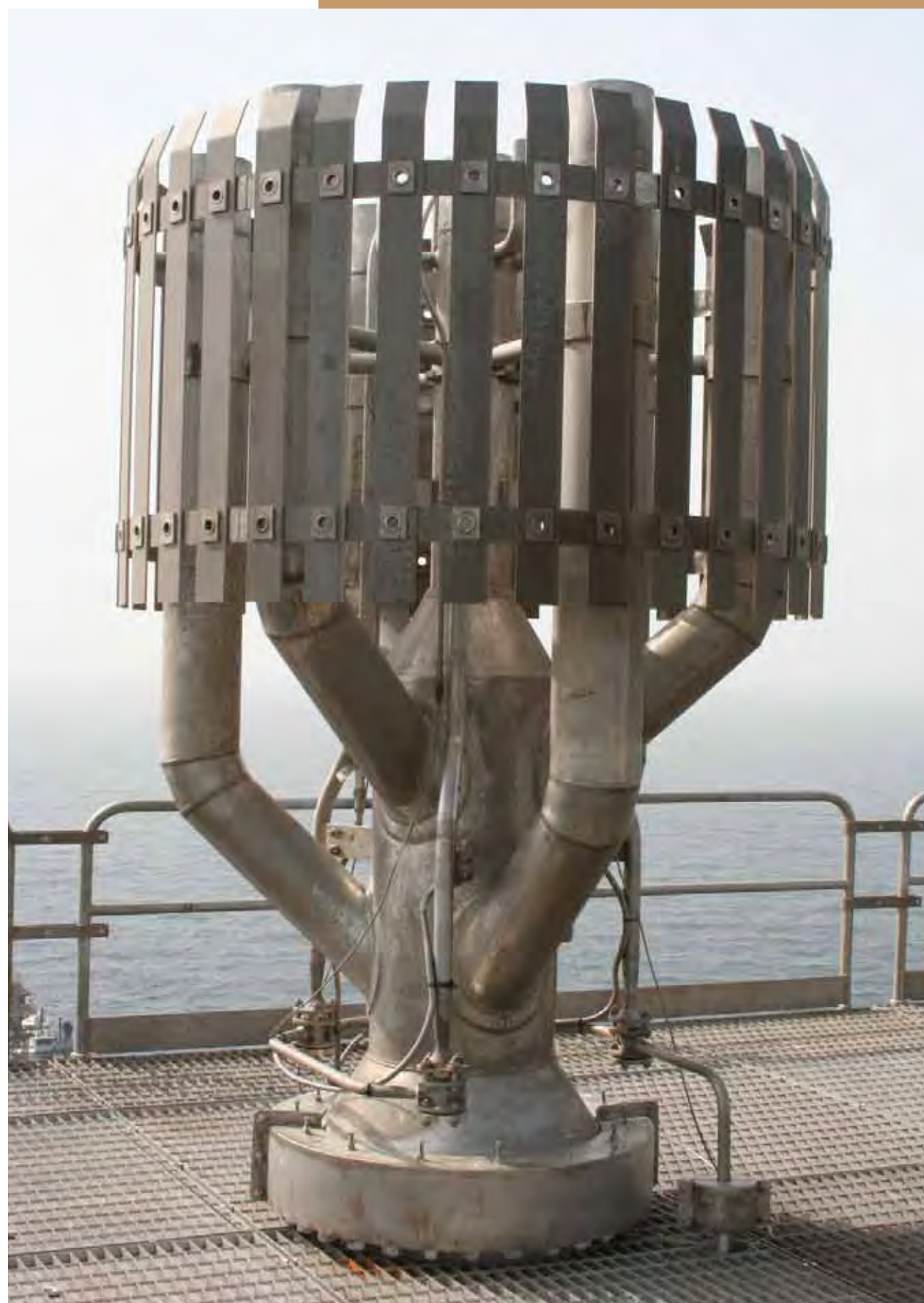
CSF-7-8 HP Flare Tip Offshore Qatar
