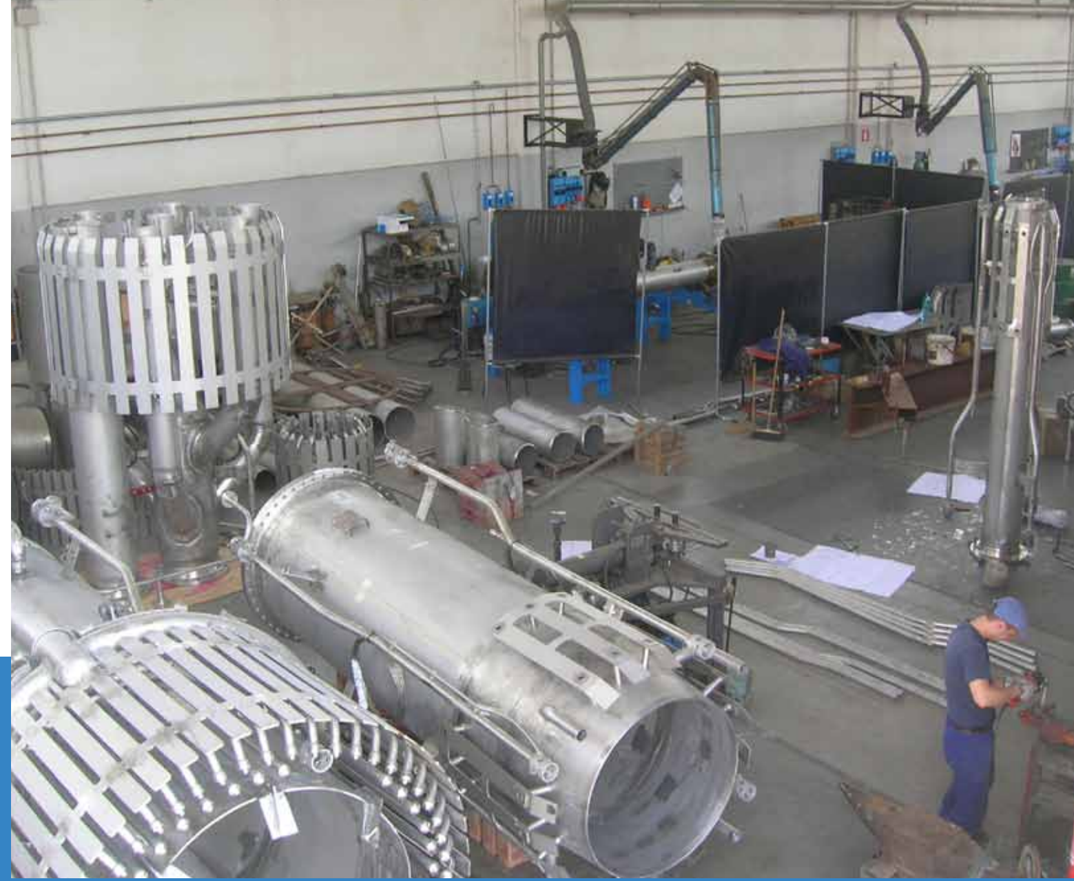
Flare Tips in GBA's dedicated stainless steel shop
